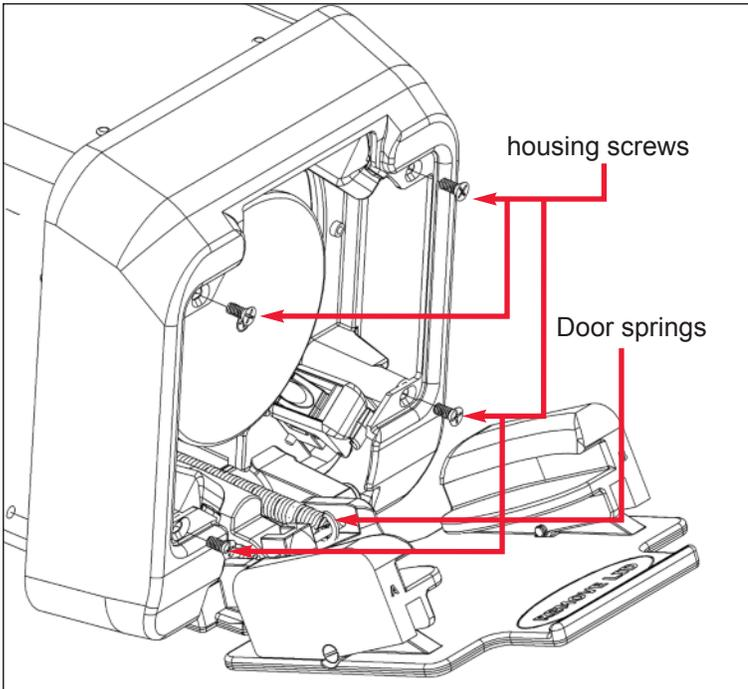
Over time “lid dust” or other debris may need to be removed from the LidSaver to keep its appearance as fresh and clean as possible. Follow these simple steps as needed.
